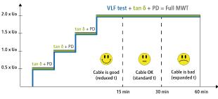
cable insulation. Moreover, a partial discharge measurement shows and locates the PD faults precisely. The highlight of MWT is the condition-based test duration: Provided it is permitted, the test duration can be shortened, which in turn lowers costs. This way, the cable is only exposed to the increased test voltage for the required duration.
